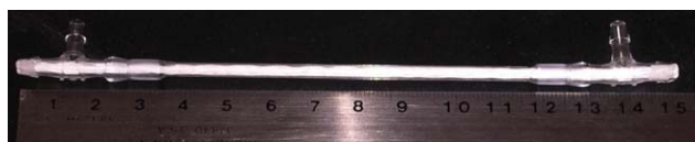
Figure 2. Mini-module used for fluorescence imaging, showing polycarbonate housing and fibers, with UV curable epoxy for potting material. Approximately 30 fibers, 15 cm in length, provide the mini-module with about 15 \text{ cm}^2 of surface area. [Color figure can be viewed in the online issue, which is available at wileyonlinelibrary.com .]
